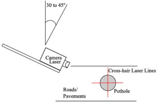
Fig. 2. Cross-hair laser pattern to detect pothole and uneven surfaces.
